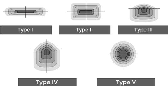
The variable optic system allows for the designer to create hybrid distributions for precise lighting requirements.
