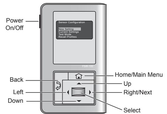
The FSIR-100 is a convenient handheld remote tool for sensor setting. Adjustable settings can be changed as needed for specific applications.
