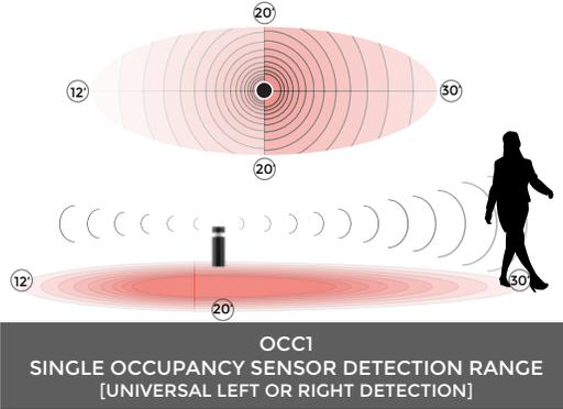
\* The integrated, smart occupancy sensor can be programmed on site to function in a variety of ways.
