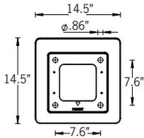
**Anchor Bolt Base Mounting Detail**
