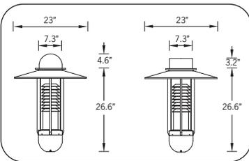
A decorative post top lantern with excellent downward symmetrical light distribution. Luminaire using energy saving COB LED lamps. Designed for lighting of entrances, footpaths and car parks.
