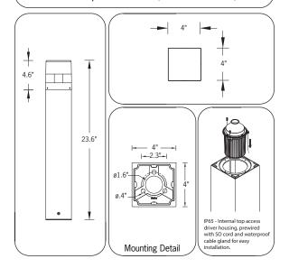
The innovative reflector technology of the Lightsoft bollard guarantees a high degree of efficiency and optimal visual comfort. Lightsoft has been developed to have excellent controlled downward light providing wide spacing ratios. It has three light shield accessories with different light distributions. The Lightsoft is available in a cylindrical or square shape design with two
