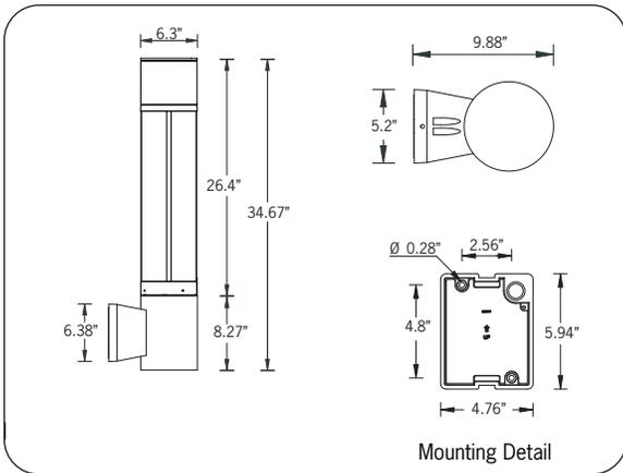
A decorative cylindrical shape wall lantern with symmetrical light distribution. Developed to compliment the Arizona light column. Low copper content die-cast aluminum housing with high corrosion resistance. Stainless steel screws. Durable silicone rubber gasket and clear impact resistant UV stabilized polycarbonate diffuser. Housing is treated with a chemical chromated protection before powder coating, ensuring high corrosion resistance. Integral control gear.
