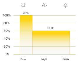
Time & dimming settings are set with the remote solar charger programmer
