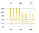
Dimming levels adapt to low voltage battery conditions
